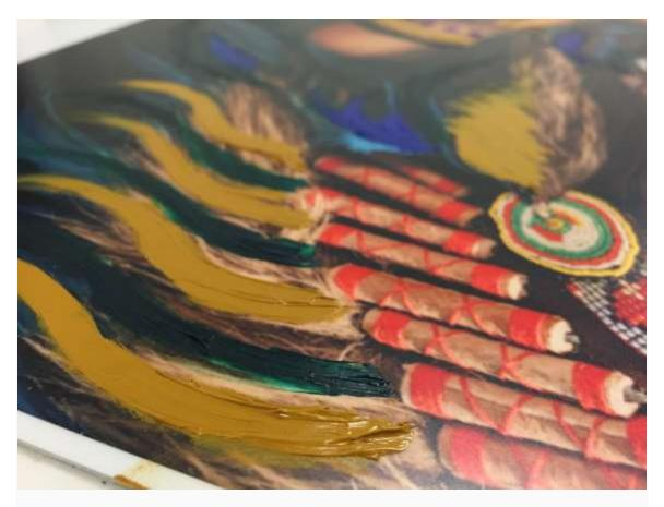
This oil-based test was done yesterday and yet the oils are still wet to the touch. As you can see from the close up detail shot, the oils sit on the surface of the laminate and don't absorb.
