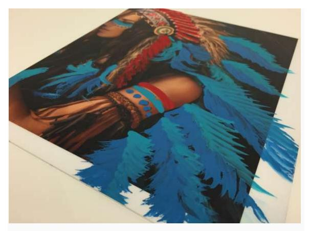
To best show you the pooling, I saturated the bright blue in this shot with a lot of water, and you can see how it beaded and pulled away from the laminate.
